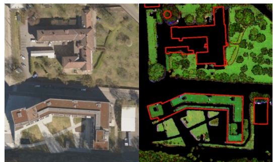
Figure 2 Identification of green roofs.
